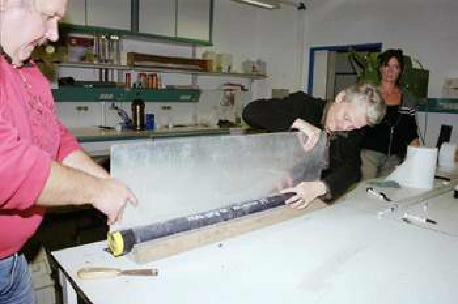
Cutting the core with a metal plate and dividing it into two halves
