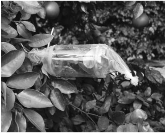
Figure 10.2 An exclusion cage designed for assessing impact of coccinellids and other natural enemies on aphids and psyllids infesting expanding grapefruit terminals. The cage is constructed from a clear plastic 2-litre soda bottle with mesh sleeves attached to either end with silicone and fastened to the branch with a length of wire secured to the inside of the bottle with packing tape. The sleeve mesh can be selected to permit the passage of particular insects (in this case, parasitoids), while excluding larger ones (coccinellids). The basal sleeve is attached tightly around the branch with a zip tie; the terminal sleeve is sufficiently long to permit unimpeded growth of the shoot for 2–3 weeks and can be untied to permit periodic access and counting of insects (photo: J.P. Michaud). (See colour plate.)
