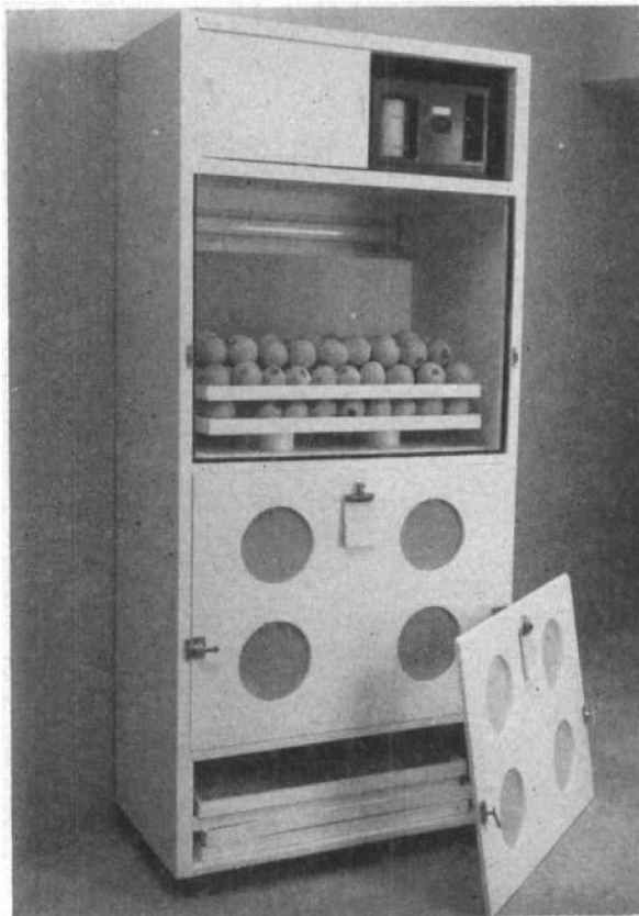
FIG. 5.— Stethorus rearing unit. The upper cage contains developing predator larvae, and the closed lower cage contains an oviposition unit.
