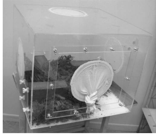
Fig. 2. Modified rearing box used in mass rearing of Sasajiscymnus tsugae at Clemson University's insectary, Clemson, South Carolina.
