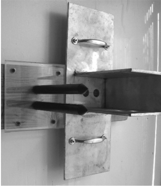
Fig. 3. Press used to make holes in wet foam blocks placed in modified rearing boxes at Clemson University's insectary, Clemson, South Carolina.
