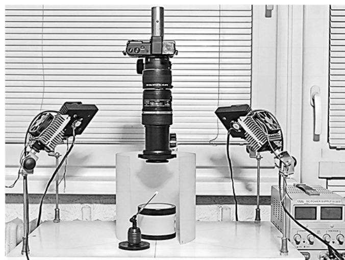
Fig. 3. Copy stand with optical equipment, diffuser, light table, and transformer (right) for operation of led lights. From top down Nikon 1-V1 camera, Nikon FT-1 adapter, Kenko TCx2 teleconverter, Tamron 90 mm macro lens (fully extended), Raynox DCR-250 super macro lens. Foreground: specimen manipulation tool.
