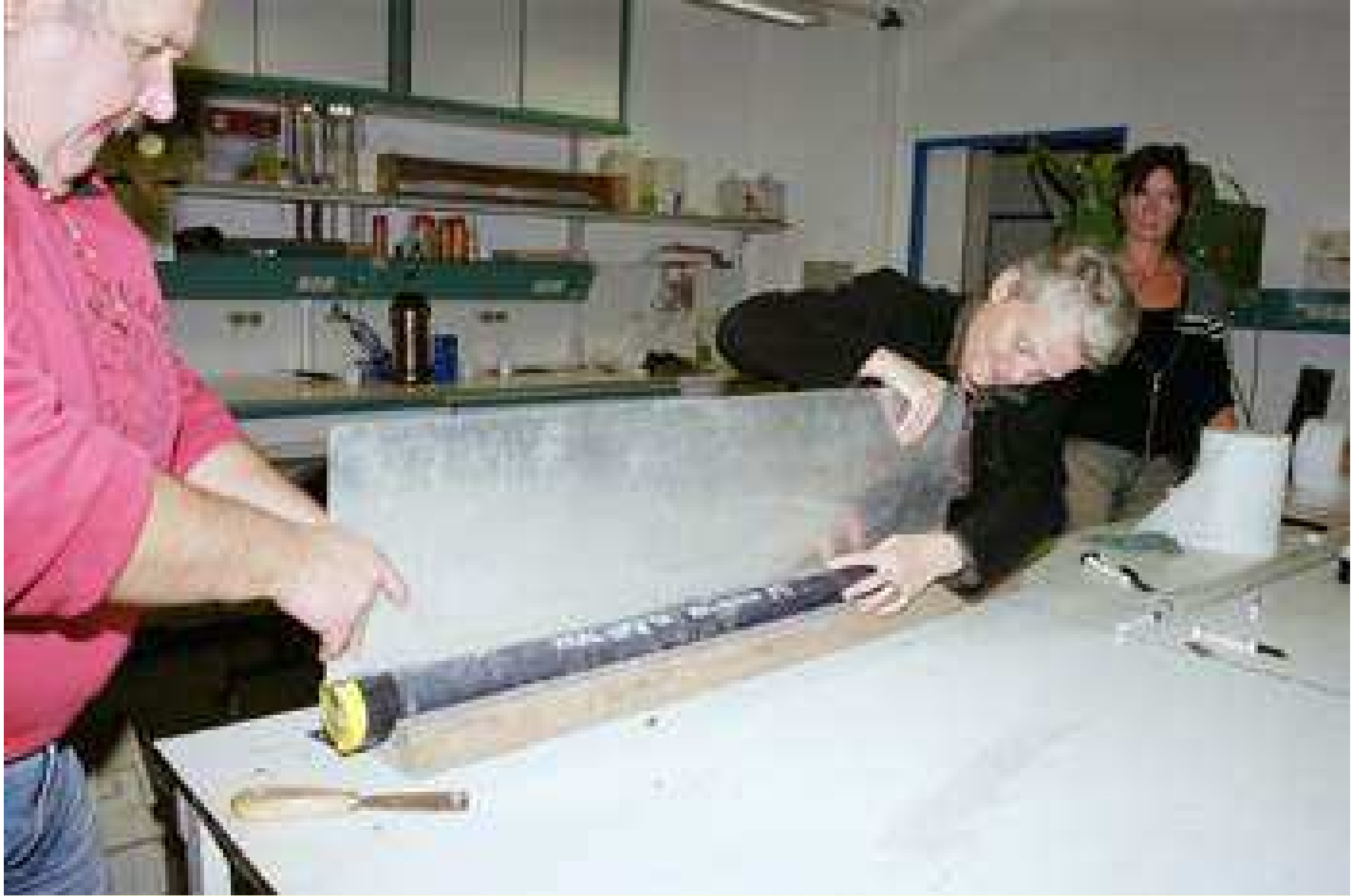
Cutting the core with metal plate and splitting into two halves
