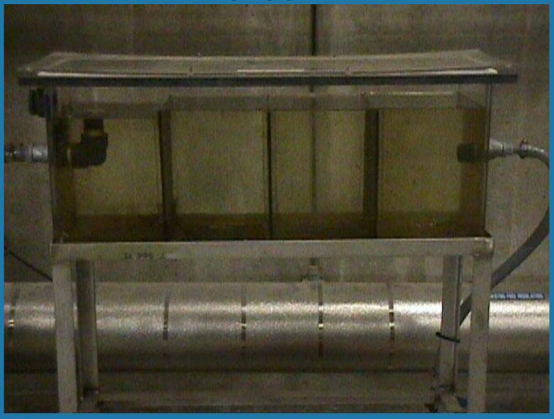
Corrosion Coupon Panel
