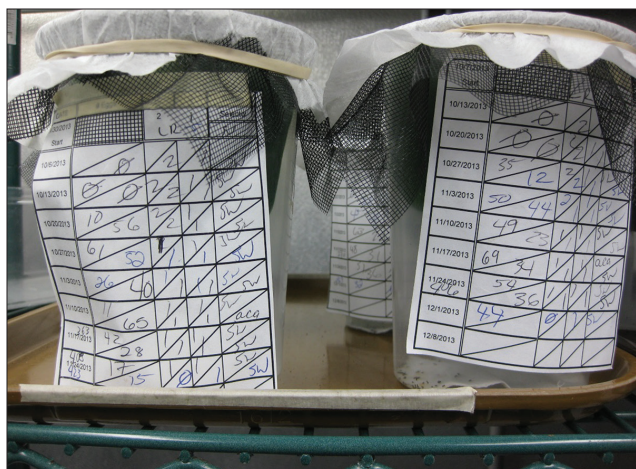
Figure 4. Emerald ash borer rearing enclosures showing screen and filter paper lids secured for oviposition. Tracking egg production data is useful for optimizing colony demography. A simple data sheet, visible on side of cup, records the day of beetle emergence, weekly egg production, and the number of beetles dead at each provisioning with new foliage. (Photo credit: Jonathan Lelito, USDA APHIS PPQ)
