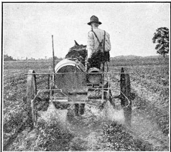
FIG. 3.—Traction sprayer with nozzle arrangement for side spraying, of type useful for spraying beans for the bean ladybird.
