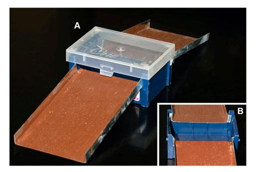
Figure 2. Assembled ramp trap with (A) lid on and (B) lid off to show notches cut into VWR pipette-tip box to receive ramp ends. During deployment, fluid is filled to approximately 2 cm.
